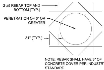
**3 TANK COVER PAD MANHOLE OPENING DETAIL**
